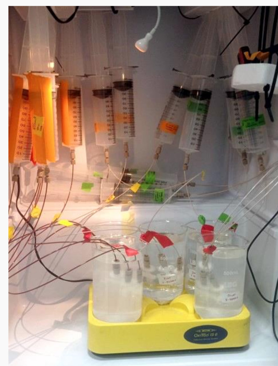
Figure 1: Experimental setup to assess the water collected by the TIMFIE device over 24 h
